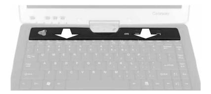
**13** With a small Phillips screwdriver, remove the four keyboard screws and put them in a safe place.
